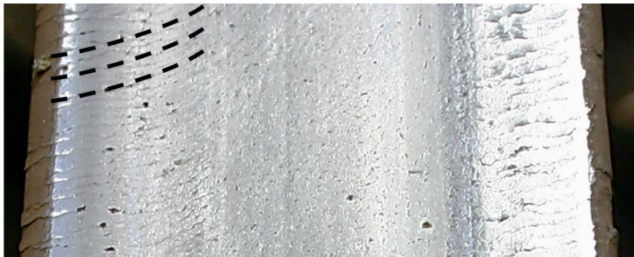
Figure 3. Commonly occurring RCF defects on the gauge corner of rails. Dashed lines highlight the curvature of the head checks from the gauge corner into the running band.
