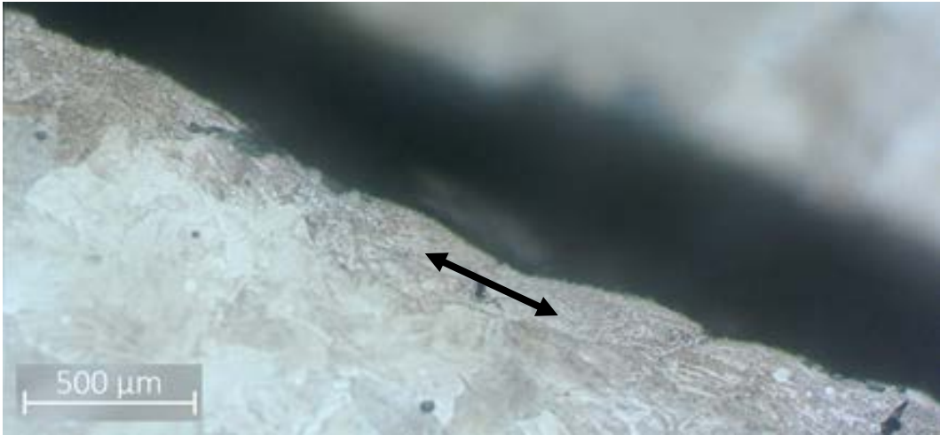
Figure 16. OM image of pearlite colonies deformed along the crack face.
