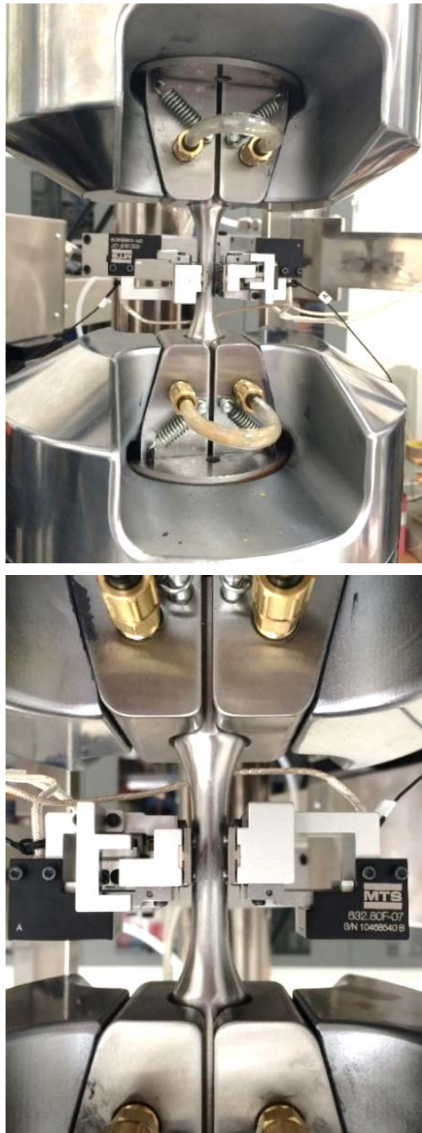
Figure 15. Experimental set-up for LCF damage initiation tests.
