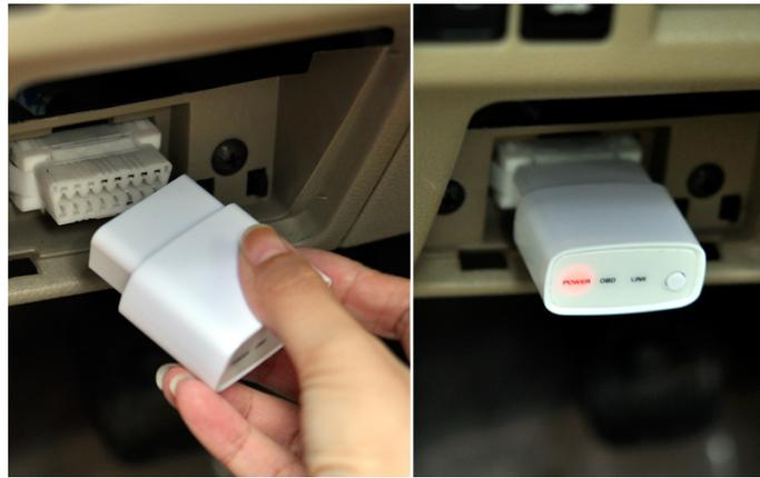
**Figure 6.5:** Connecting an OBD dongle to the OBD II port [91]
