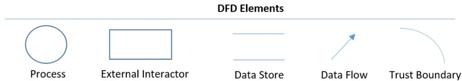
**Figure 5.6:** Common elements of a data flow diagram
