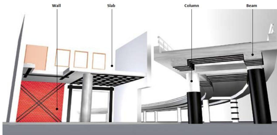
Figure 3.6 Different possibilities and areas where FRPs can be used for strengthening [10].
