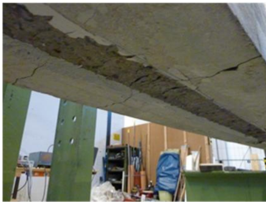
Figure G.4 Debonding of the laminate in strengthened beam with unprestressed laminate.
