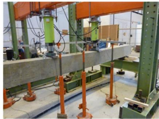
Figure G.4 Debonding of the laminate in strengthened beam with unprestressed laminate.
