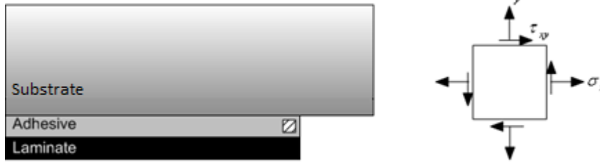
Figure 3.12 Illustration of shear and normal stresses in the adhesive layer [9].
