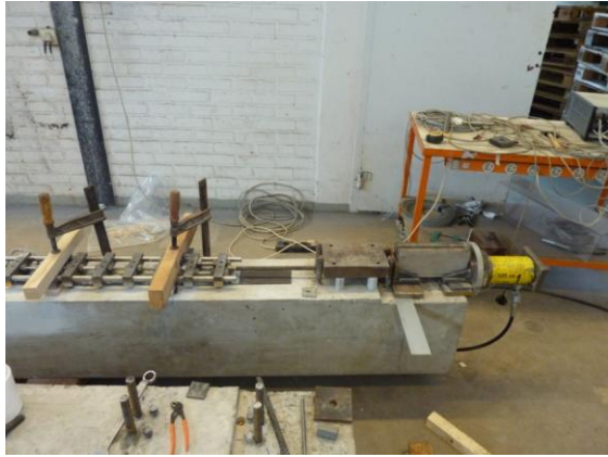
Figure 7.2 Test setup with hydraulic jack mounted and using clamps to hold the device in place.
