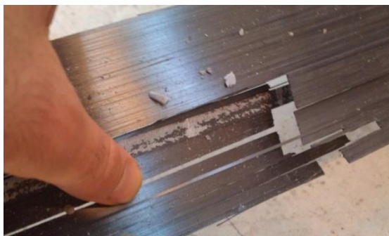
Figure G.5 Failure by laminate rupture in the strengthened beam with 85kN prestressing force.
