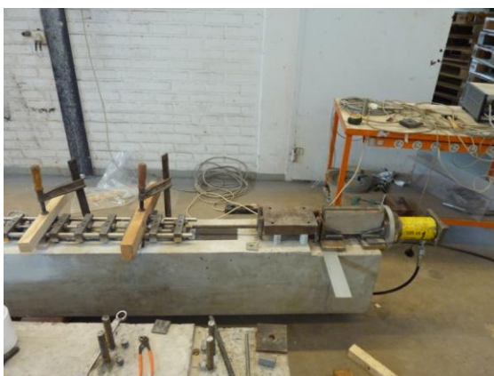
Figure G.2 Test setup with hydraulic jack mounted and using clamps to hold the device in place.
