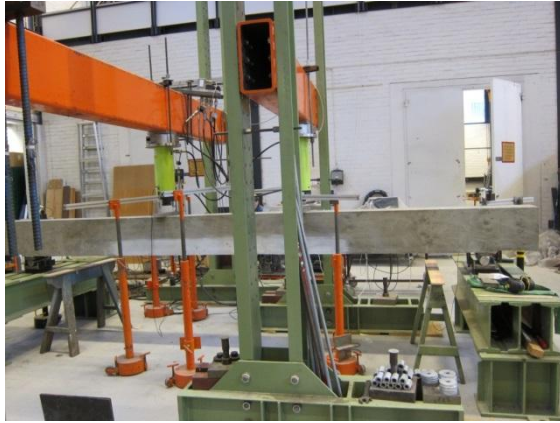
Figure G.3 Test setup with four-point bending that was used.
