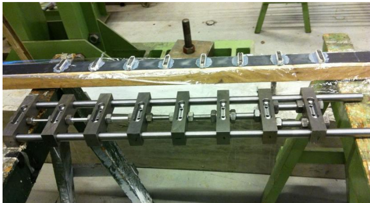
Figure G.1 Picture showing the first prototype of the prestressing device together with the CFRP laminate with adhered steel tabs.
