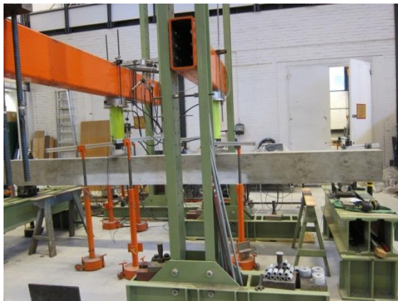
Figure 7.3 Test setup with four-point bending that was used.
