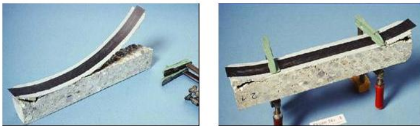
Figure 4.7 Laminate debonding caused by high shear stresses at the laminate end as a result of prestressing [34].
