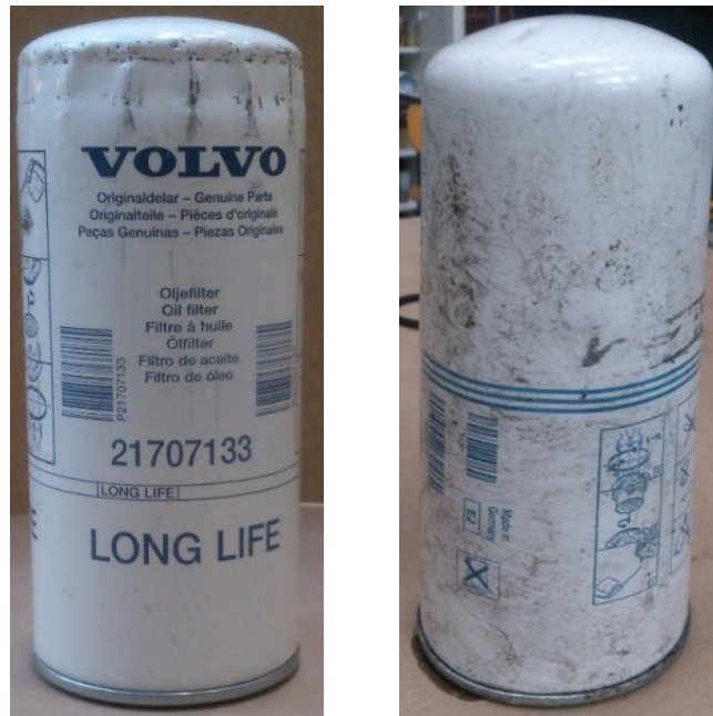
Figure 19: Filters collected from recycling dumpster at the service provider. Note the dents from the filter wrench in the left image and the grease and dirt on both filters
