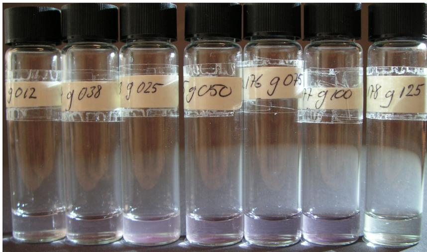
**Figure 69:** Photograph showing solutions of nitric acid, triton X-100, carbowax, deionized water and different amount of gold colloids containing 5 nm GNPs
