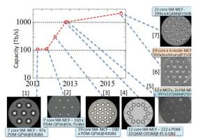
Fig. 1: High-capacity MCF transmission experiments
