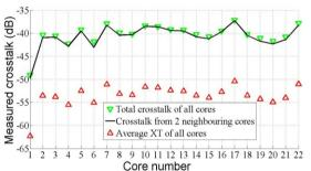
Fig. 3: Measured core-wise IC-XT for 22-core fiber
