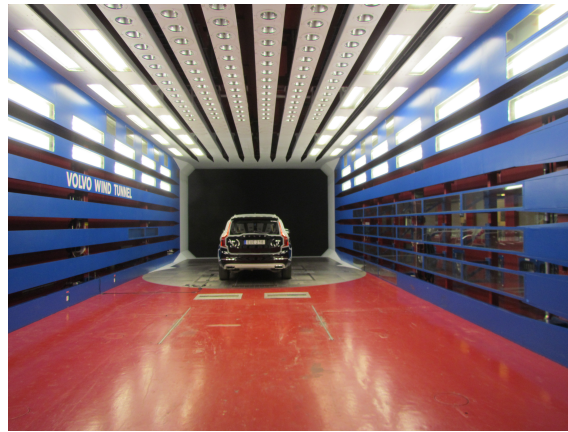
Figure 3.8: Overview of the Volvo wind tunnel with Volvo XC90.
