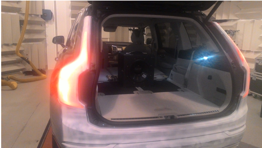
Figure 3.7: Position of sound source inside the car.
