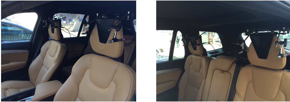
Figure 3.3: Microphone positions on the front and rear seats.
