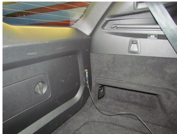
Figure 3.4: Accelerometer mounted on the tailgate.
