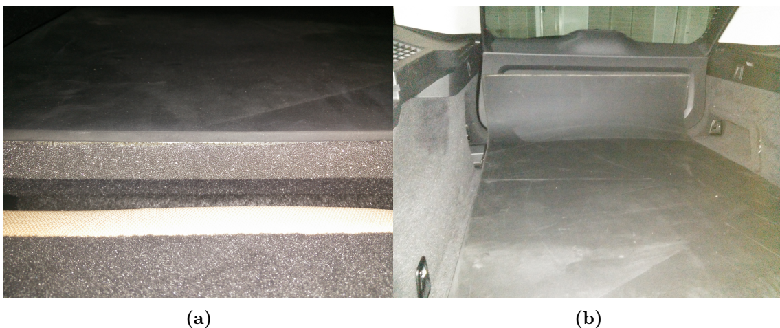
Figure 4.10: Heavy layer covering the tailgate
