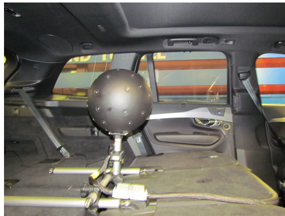
Figure 3.9: Position of 3D-CAM inside the car.
