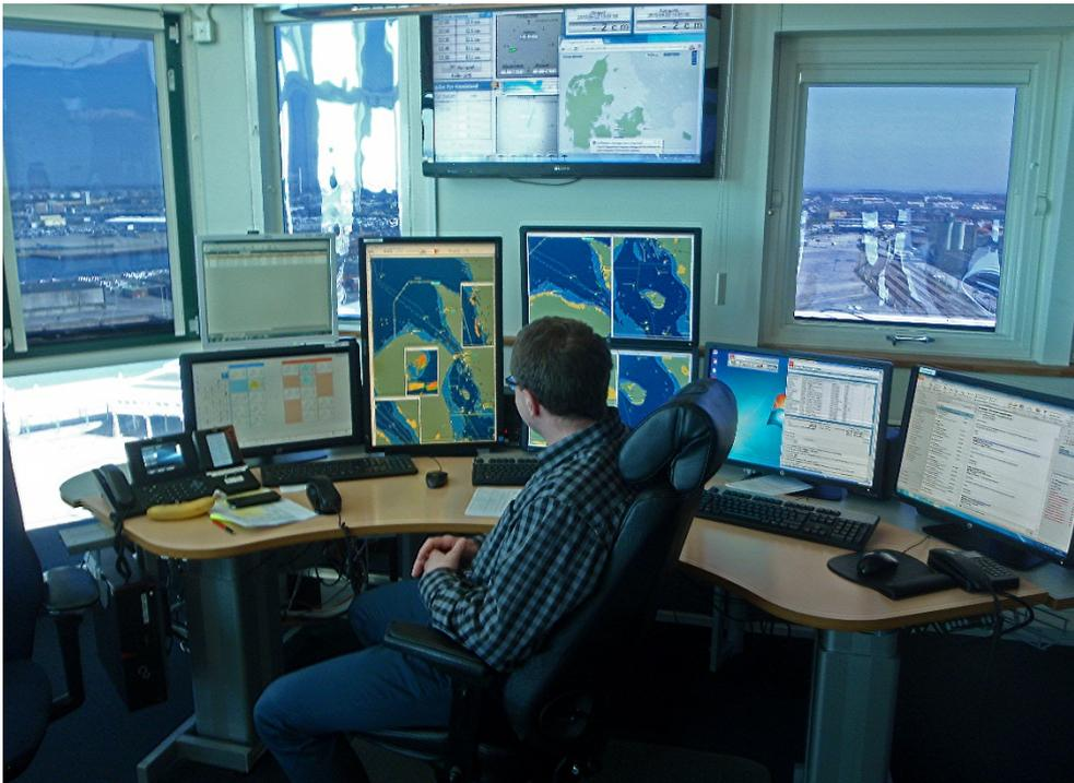
*Figure 16. VTSO at work, showing VHF radio (left), chart displays (centre), email/ship reporting (right) and weather (top).*
