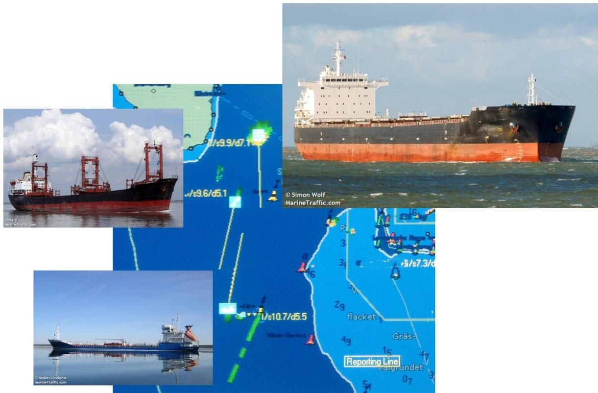
Figure 12. VTS screen (centre) showing close quarters situation between vessels (vessel images: MarineTraffic.com).
