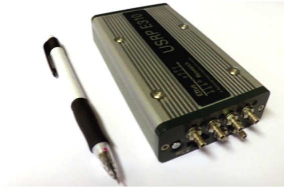
Fig. 2 Photo of the USRP E310 together with a pen for better illustration of the dimensions of the device.
