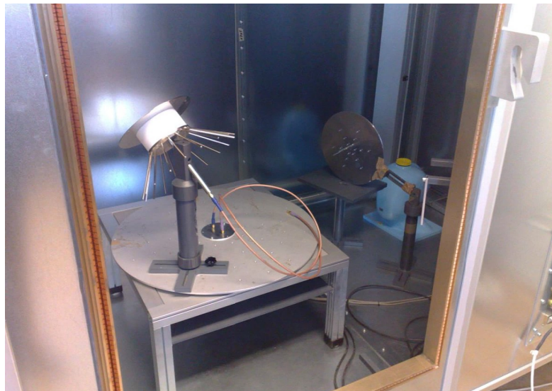
Figure 4.5: The disk-cone antenna as reference in the reverberation chamber
