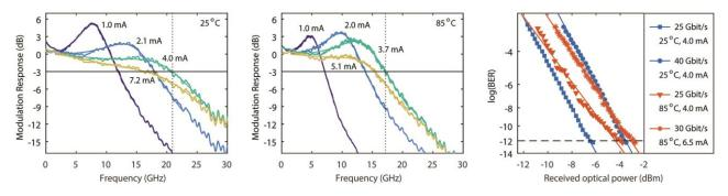
**Fig.3** Left and middle: Small signal modulation response at 25 and 85°C. Right: Data transmission at 25 and 40 Gbit/s at 25°C and 25 and 30 Gbit/s at 85°C.
