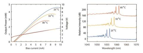
Fig.2 Left: Output power and voltage vs. current at 25, 55, and 85°C. Right: Emission spectra at 4 mA.
