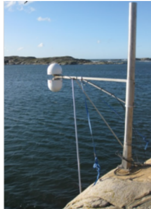
Figure 4.2: Onsala's GNSS tide gauge. The figure was taken from Figure 5 in (42).
