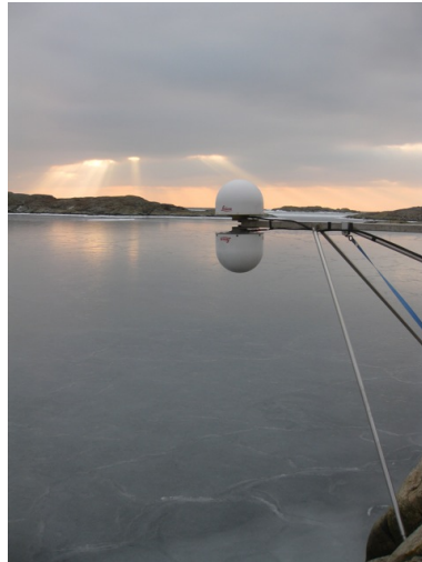
Figure 4.3: Onsala's GNSS tide gauge with ice during February 2012 (doy 37).
