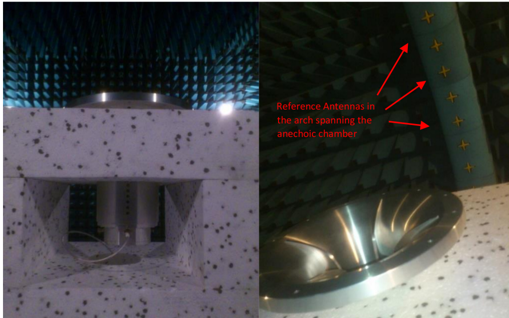
Figure 5.9: Scaled Band 1 feed prototype in the anechoic measurement chamber, the yellow crosses are the reference antennas that span the arch around the feed. Walls are covered in absorbing material to minimize unwanted reflections.
