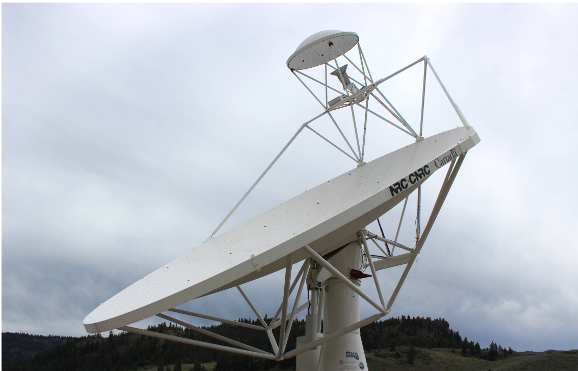
Figure 5.30: The Sep2015 feed prototype mounted on the DVA-1 dish at the DRAO site, Penticton, B.C., Canada. The feed is seen just underneath the SR.
