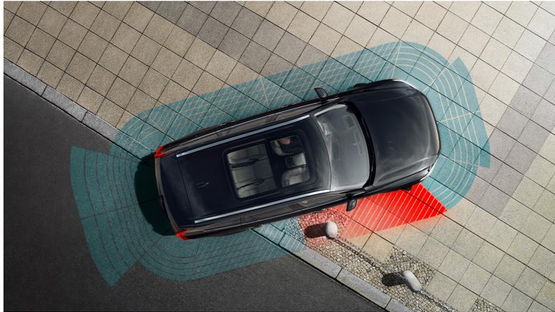
**Figure 1.1:** Field of view for the on-board sensors that sense the immediate vehicle surroundings. These sensors are used in e.g. driver assistance functions such as semi-automatic parking and collision warning [7].
