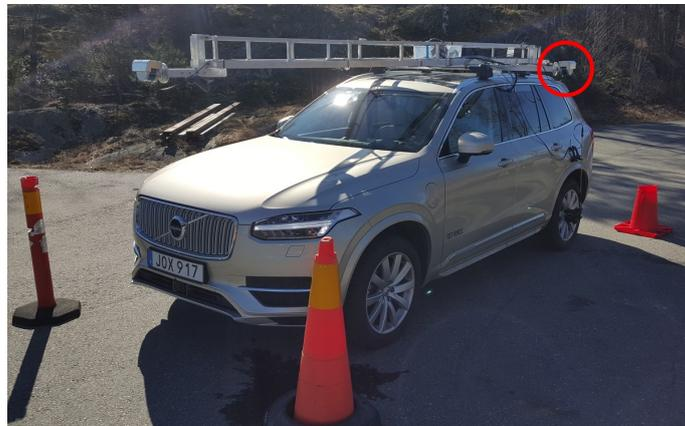
(b) The lidar system mounted on a vehicle. The left side lidar is circled.
