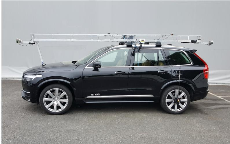
**Figure 1.5:** The test vehicle used in this thesis work. The reference system is built by Volvo Car Corporation and used for verifying the vehicle’s on-board proximity sensors. The proximity sensors’ field of view is shown in Fig. 1.1. The reference system is mounted on top of the vehicle and includes four lidars, one placed on each side of the car.
