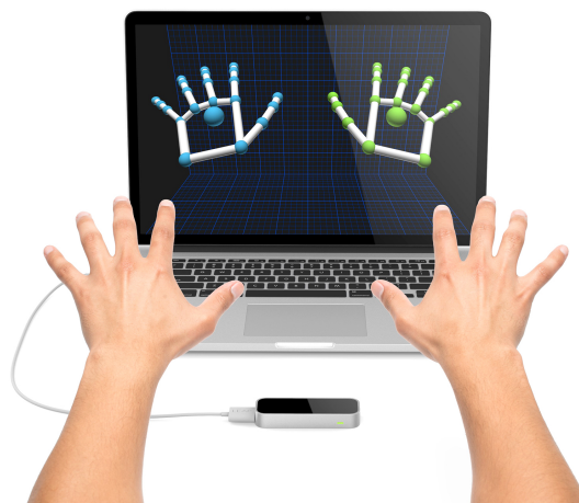
Figure 2.3: Visualization of a Leap Motion sensor setup. [37]
