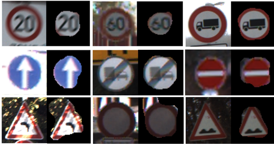
Figure 3.5: Examples of segmented images from GTSRB. From left to right and top to bottom: samples from classes “0”, “3”, “16”; “35”, “42”, “17”; “19”, “15”, “22”.
