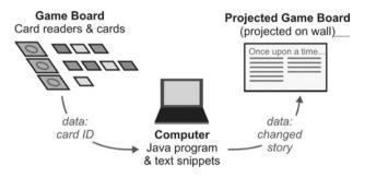
Figure 33: An overview of the components and the dataflow in myTHeme
