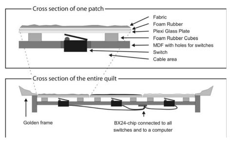
Figure 4: The construction of the Interactive Quilt.
