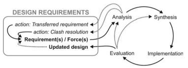
Figure 24: One iterative cycle in one design discipline.
