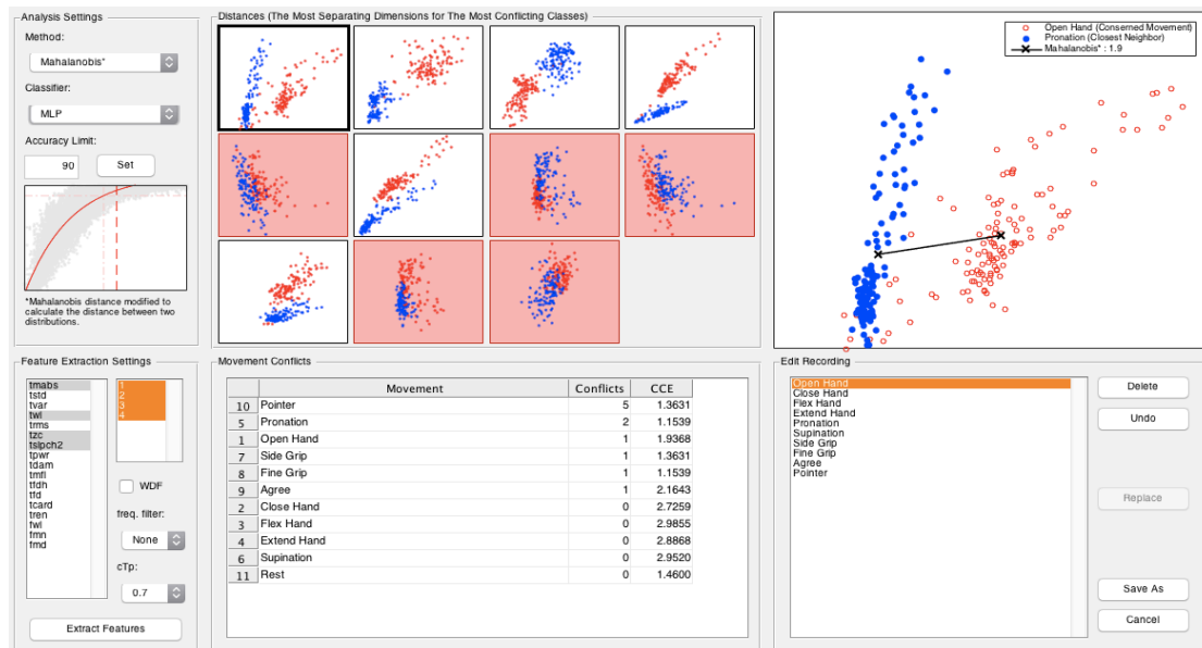
Figure 16: A screenshot of the data analysis tool of BioPatRec. Showing a recording of a hand performing 10 movement plus rest.
