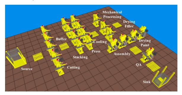
Figure 6-2: Delmia Quest model of manual baseline process for the A350 scenario
