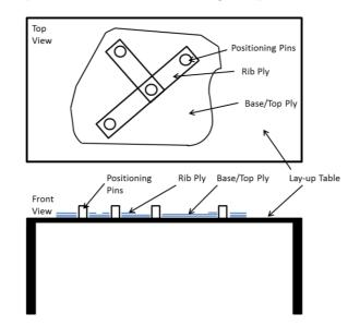
Figure 5-7: Template with pins to position plies and TFPs via holes cut during NC ply cutting
