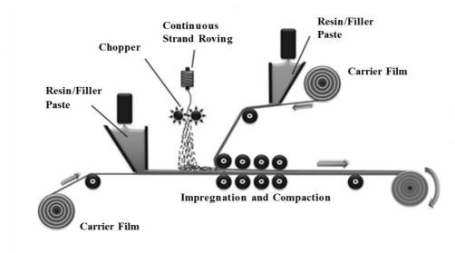
Figure 2-2: Schematic view of the production of SMC (adapted from Fette M. et. al., 2015)
