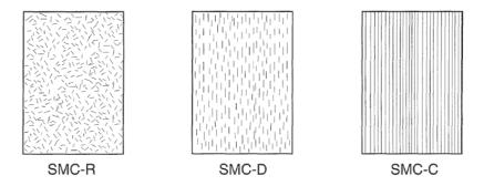
Figure 2-1: Different length and direction of fibres in SMC (Berthelot, 1999)
