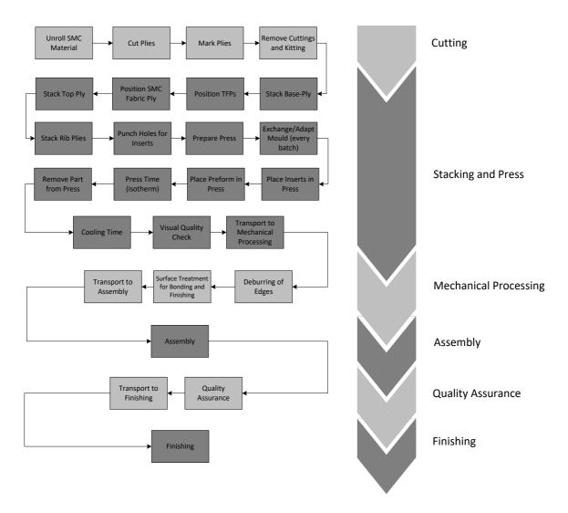
Figure 4-3: Flowchart of the sidewall production chain including assembly and paint
