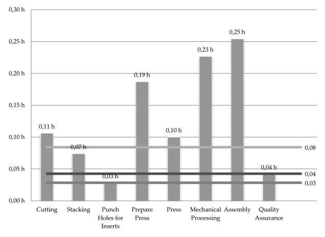
Figure 10-9: Cycle time chart of human-machine allocation approach
