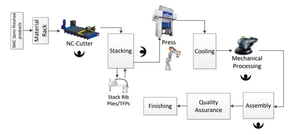
Figure 5-11: Conceptual line type layout for lean manufacturing approach
