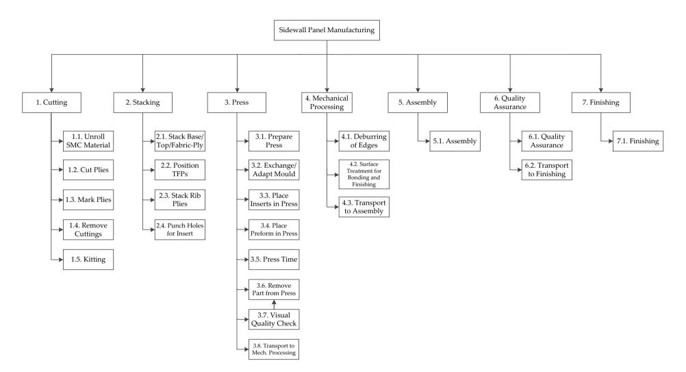
Figure 4-13: Hierarchical Task Analysis (HTA) of the sidewall manufacturing process
