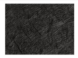
Figure 2-5: Needled airlaid fleece made of pyrolised carbon fibres (Fette M. , Wulfsberg, Herrmann, Stöß, & Rademacker, 2015)
