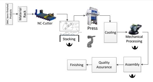
Figure 5-9: Conceptual line type layout for lean manufacturing approach
