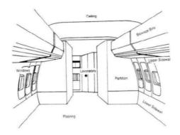
**Figure 2-6:** Aircraft interior cabin components (Committee on Fire and Smoke-Resistant Materials for Commercial Transport Aircraft, 1996)
