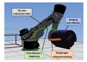
**Figure 2-12:** End effector for draping small and large dry textiles mounted at an industrial robot (Angerer, Ehinger, Hoffmann, Reif, & Reinhart, 2011)
