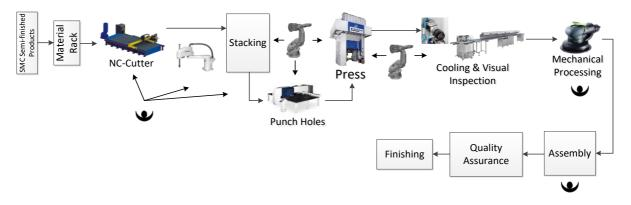
Figure 5-3: Conceptual line type layout for technocentric approach
