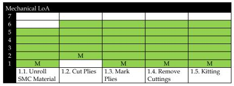
Figure 4-14: Min- and max LoAmech of the cutting operation with current levels marked with "M"
