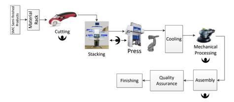
Figure 5-6: Conceptual line type layout for human-centred approach
