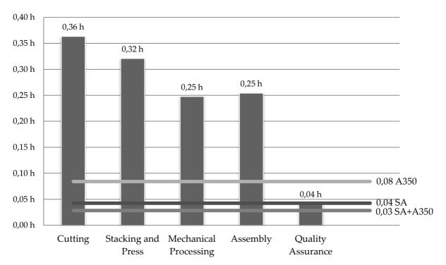
**Figure 4-10:** Plot of cycle times (bars) against the required takt times for A350, SA and SA+A350 (horizontal lines)
