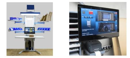
**Figure 5-4:** Innovative image recognition assistance system ("Der schlaue Klaus") (Optimum GmbH, 2016) (handling online, 2016)
