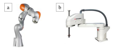
**Figure 5-10:** (a) Collaborative articulated robot and (b) SCARA robot (Robot Worx, 2016) (Softpedia, 2016)
