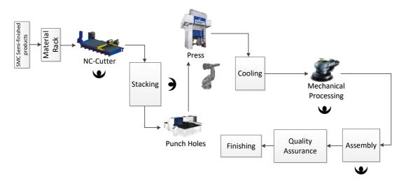
Figure 5-13: Conceptual line type layout for human-machine task allocation
