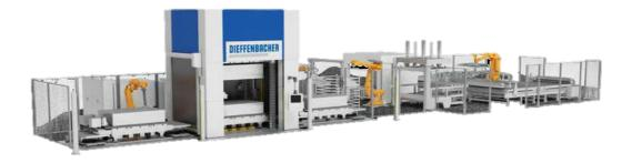
Figure 2-13: Fully automated SMC production line by Dieffenbacher (Dieffenbacher GmbH, 2015)
