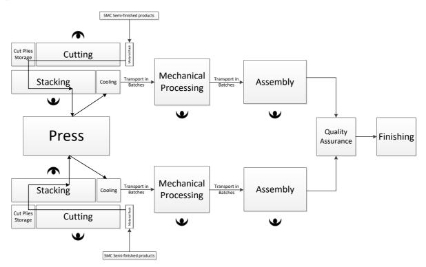
Figure 4-11: Possible layout for the baseline process based on previous
