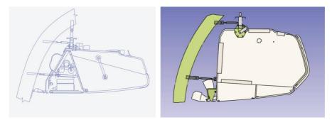
**Figure 2-8:** Illustration of a pivot bin in closed position (left) and shelf bin (right) used in Boeing aircrafts (Simmons & Worden, 2001)
