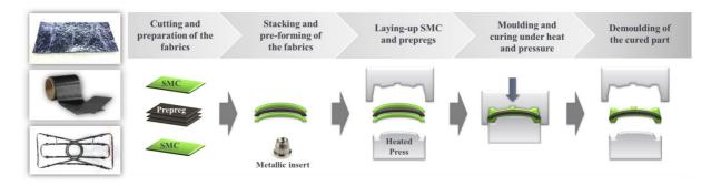
**Figure 2-3:** Compression moulding process cycle using SMC and prepreg material (Wulfsberg, et al., 2014)
