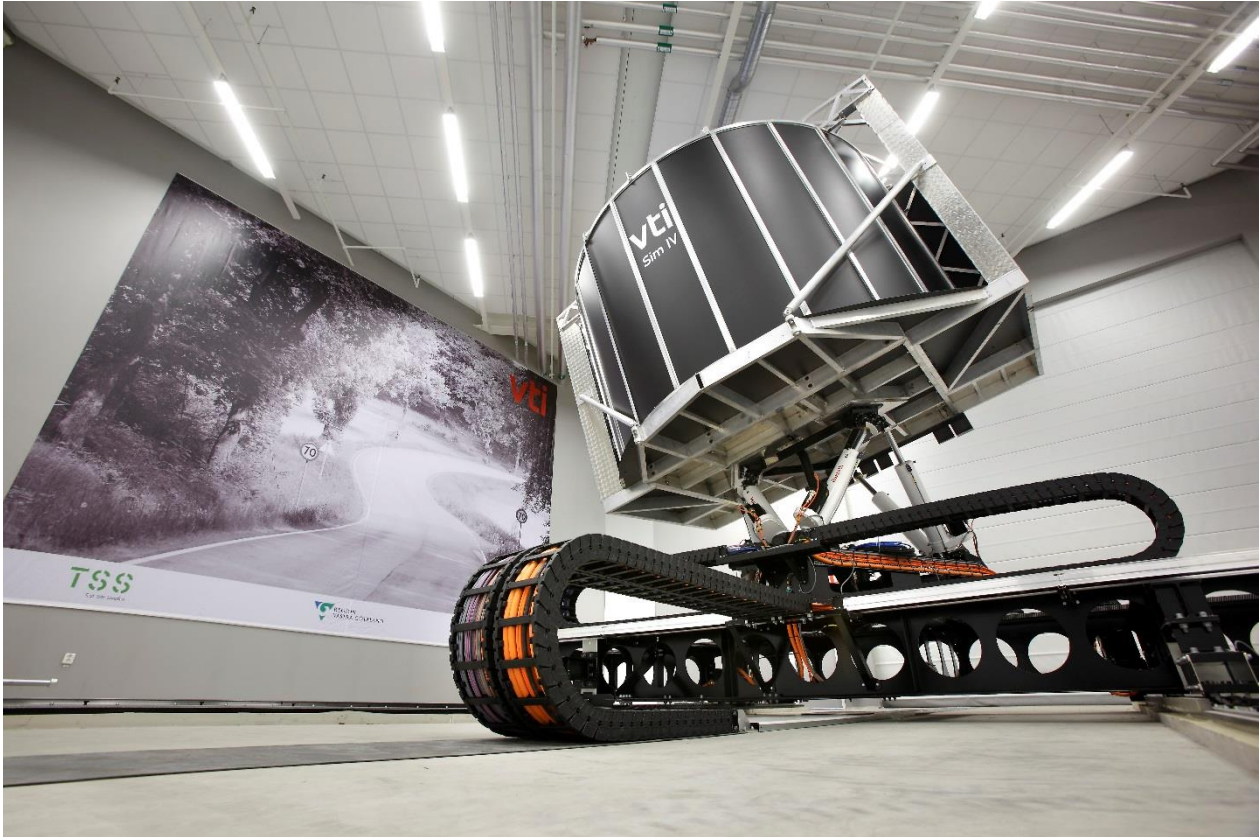
Figure 2. VTI SimIV. Hexapod with XY-sled motion platform. (Photo: Hejdlösa Bilder AB)
