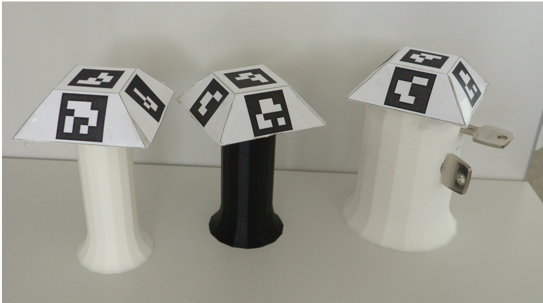
Figure 3.3.: Three 3D-printed controllers for practicing different grasps. The keys are used for pinch grasps.
