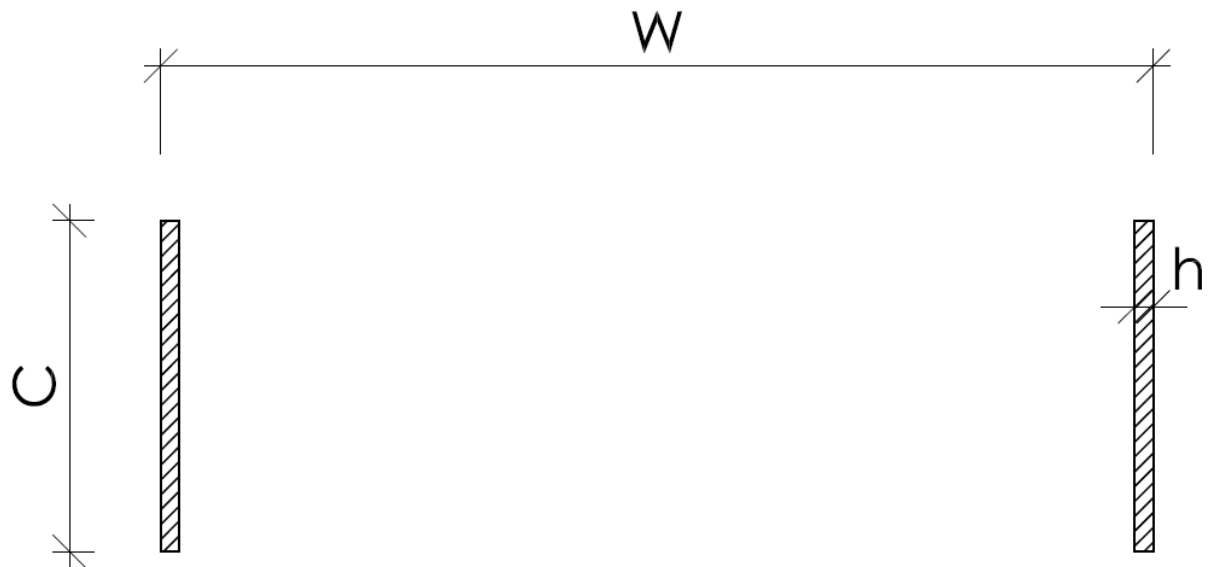
Figure 54 Perimeter system. The building width, W , is set. Then the column width, h , is calculated to achieve a maximum deformation of L/500 .
