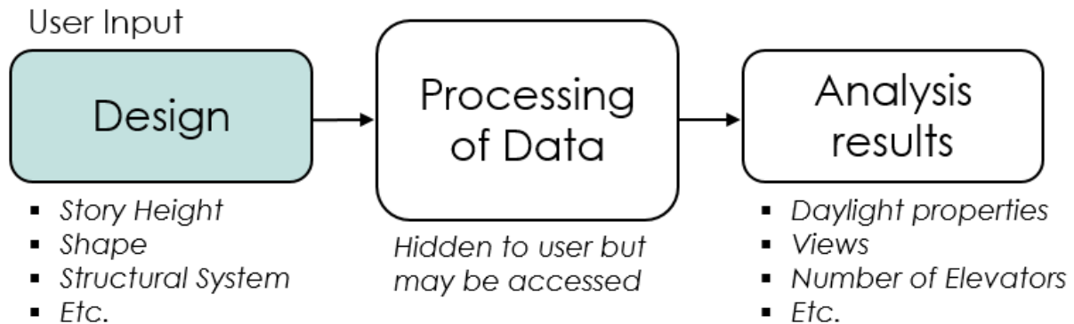
Figure 43 Schematic view of the way the design tool functions. The user inputs the design, which is processed, and the analysis results are displayed to the user
