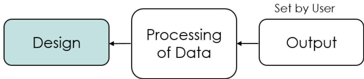
Figure 56 Reversed design process with the user specifying a desired outcome and the analysis being carried out in reverse to find what design option(s) is the best fit
