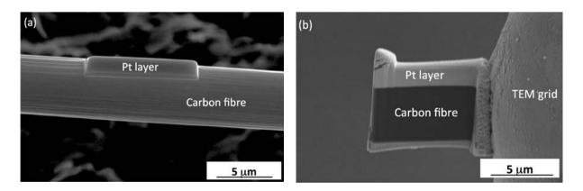
**Figure 1**. SEM micrographs showing the TEM specimen preparation procedures. (a) A carbon fibre with a Pt layer on top to protect the surface. (b) A TEM specimen with axial cross-section of the carbon fibre.
