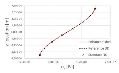
Figure 5. Normal stress distributions,  $\sigma_z$ , through the thickness of the laminate at the centre. The red solid line is the estimated stress distribution from the enhanced shell elements. The dashed black line is the distribution from the reference 3D model. The cross-marks are the stresses at the element centroids for the standard 3D model.
