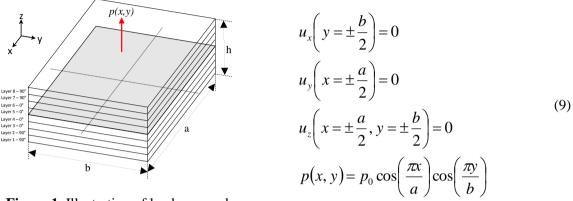
Figure 1. Illustration of load case and composite model.
