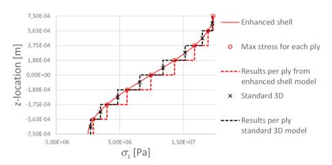
**Figure 6.** For the enhanced shell model, the normal stress distribution is marked with a solid red line, the maximum within each ply with a red circle and the extracted distribution for failure initiation with a dashed red line. For the standard 3D model, the maximum within each ply is marked with a black cross and the distribution for failure initiation with a dashed black line.
