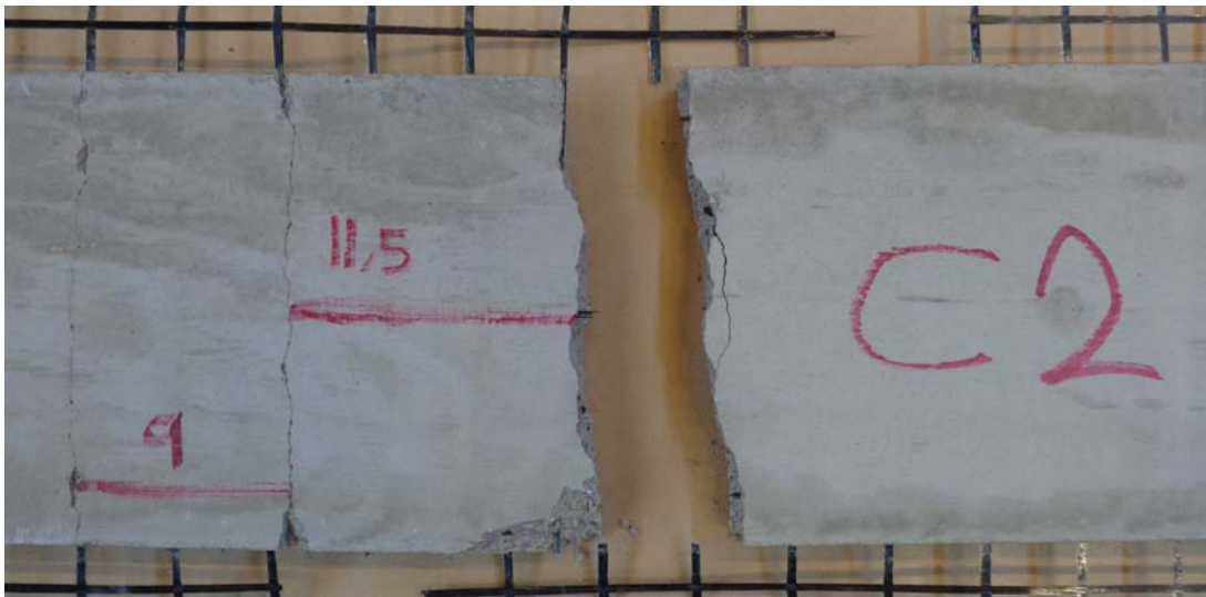
Figur 5-15 The condition of specimen number one with carbon textile and concrete mixture 2 after failure.
