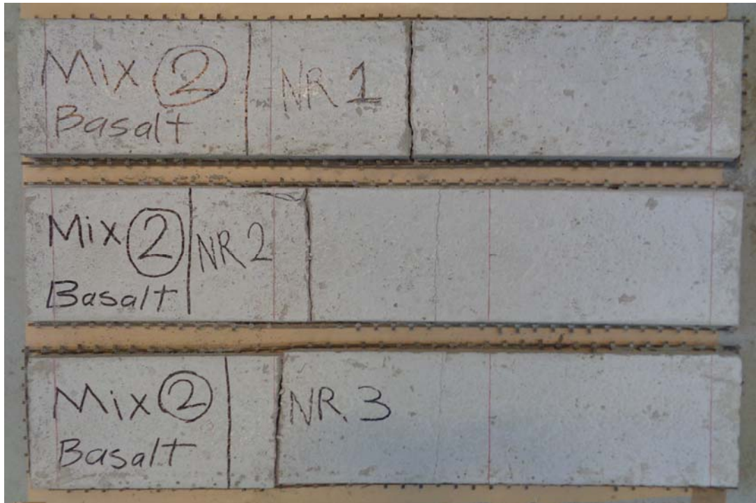
Figur 5-7 The condition of three plates with basalt textile and concrete mixture 2 after failure.
