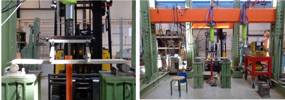
Figur 3-4 Flexural test arrangement (Photo: Ihsan Al-Khazaali).
