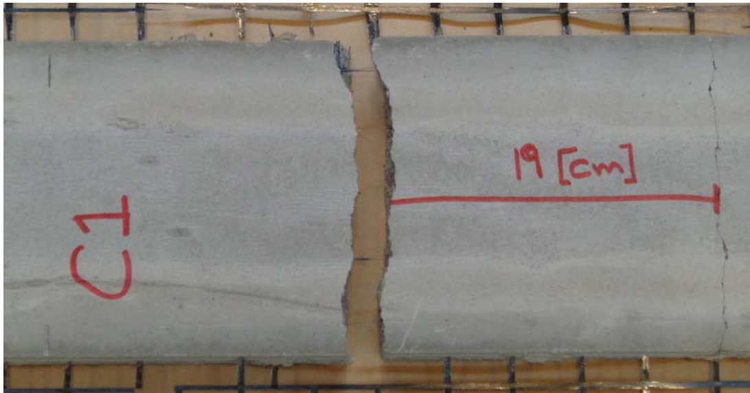
Figur 5-11 The condition of a plate with carbon textile and concrete mixture 1 after failure.
