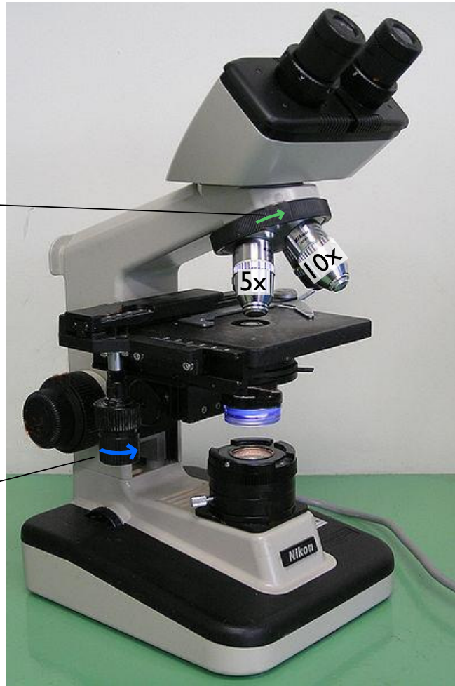
Figure 2.4: Depicting zooming and panning actions on a microscope using scale-space diagrams. The microscope's circular field of view remains the same size, but when zooming in by switching the lens it projects to a smaller area of the tissue. Photograph of microscope is used under CC-BY-SA license.
