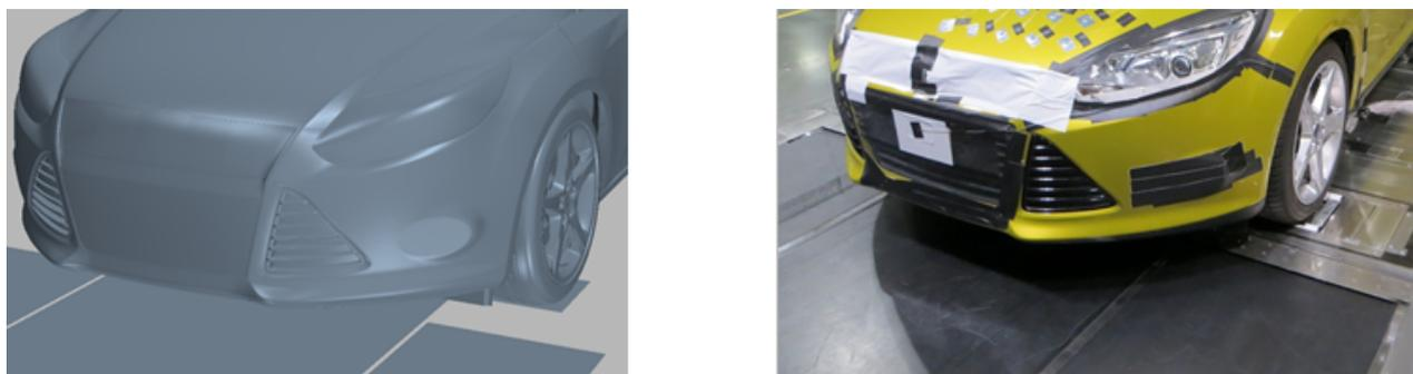
Figure 5.2: *Closed cooling - Virtual vs real*
