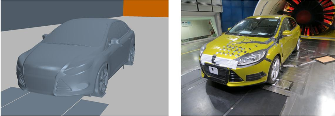
Figure 3.3: *CFD and Pinifarina wind tunnel*
