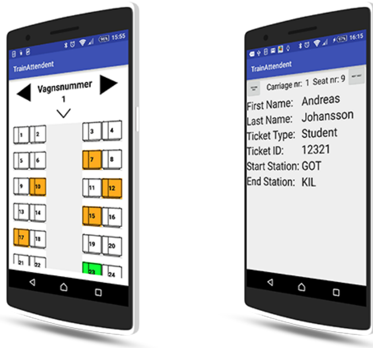
Figure 4.5: The Android application as shown on the attendant's device. Note the coloured seats in the left view: these correspond to seats with a non-vacant status. Pressing a coloured seat results in the right view, where the application displays relevant data for the seat in question.
