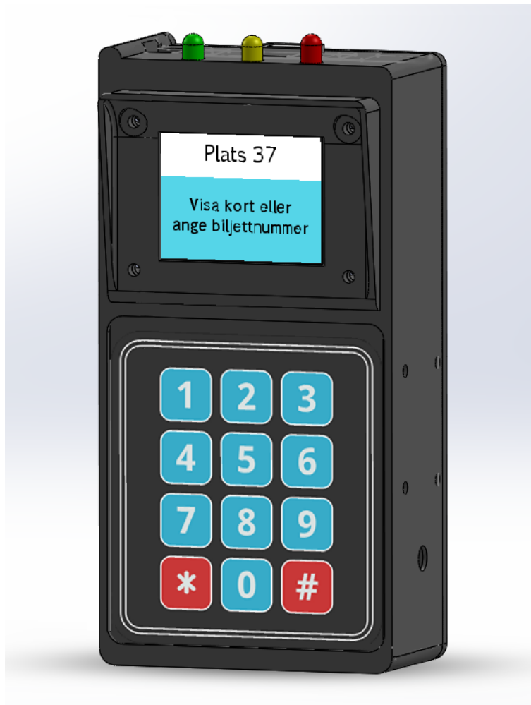
Figure 4.2: 3D-rendering of the seat unit alpha prototype. Notice the display featuring a protective screen which adds to the total thickness of the unit as seen in figure 4.1 . The holes on the right side of the unit make up an air hole for the buzzer (large hole) and mounting holes for the XBee signal converter (four smaller holes).
