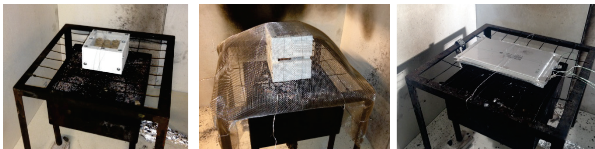
Figure 1 Experimental setup before burner start for test B (left), test C (mid) and test D (right).
