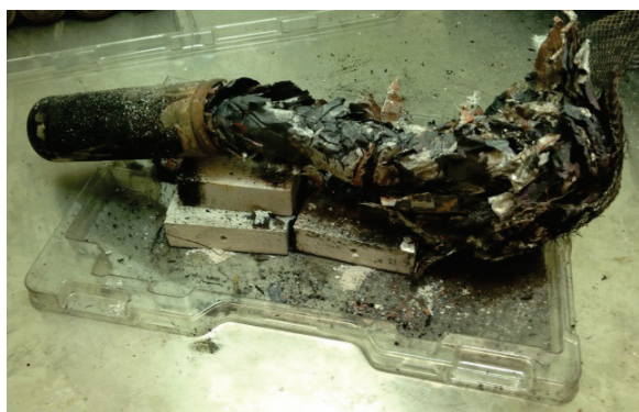
Figure 3 Results for test C, Lifetech 100% SOC. The photo is taken during tear-down analysis and showing the cell interior expelled out. The cell was caught by the steel net in the protective test box.
