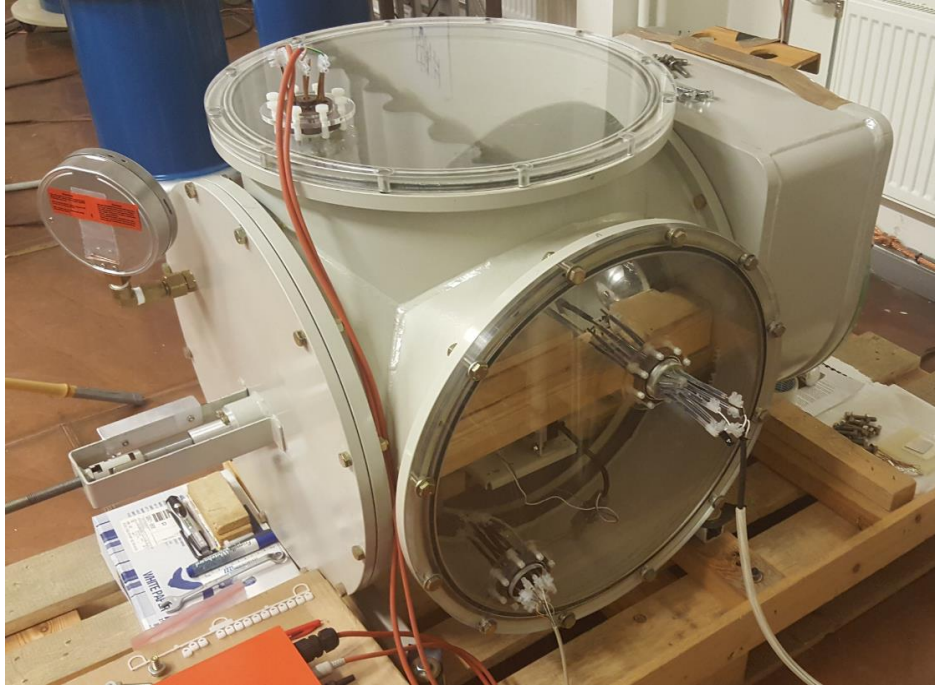
Figure 4.1. General view of the test chamber, inside which the experimental setup comprising charging arrangement and electrostatic probe is assembled.
