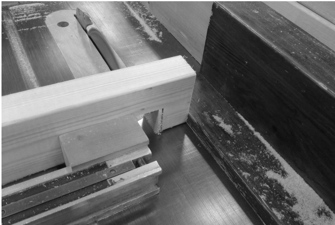
Figure 7.2 Producing a notch in a circular saw by cutting away more and more material.
