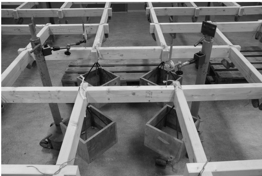
Figure 7.8 Setup for failure load test. Baskets hung to the four inner nodes and 2 kg lead weights remaining on the rest.
