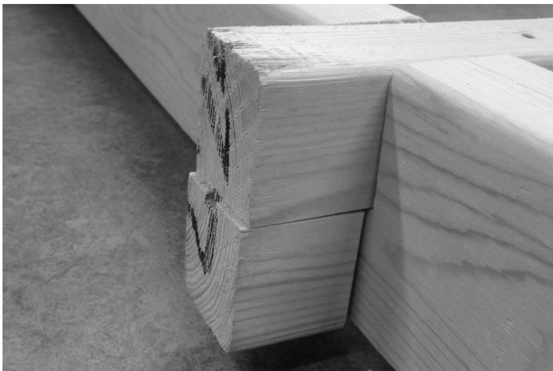
Figure 7.3 End part of one beam cracked during assembly.
