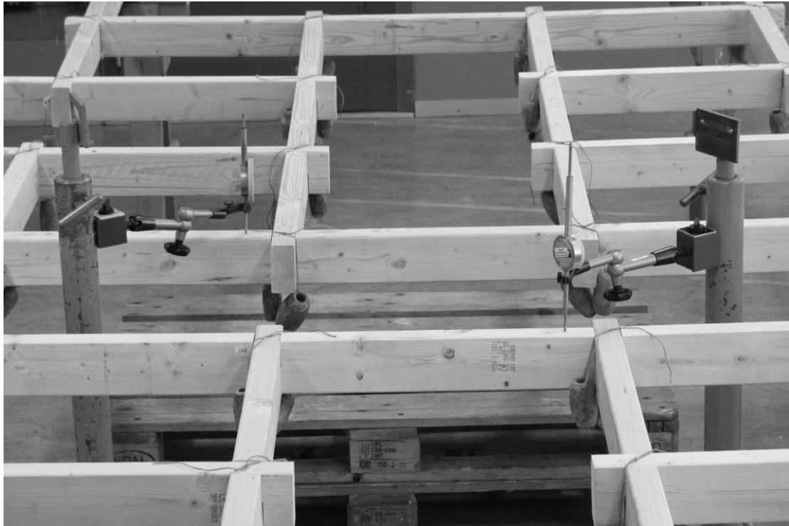
Figure 7.6 The SLS test setup with lead weights applied to all connections and deflection gauges installed.
