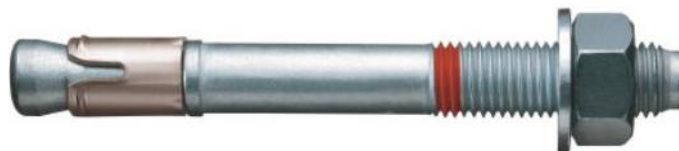
Figure 34 - The chosen expander bolt from Hilti should be with diameter 10 mm and anchoring length 90 mm
