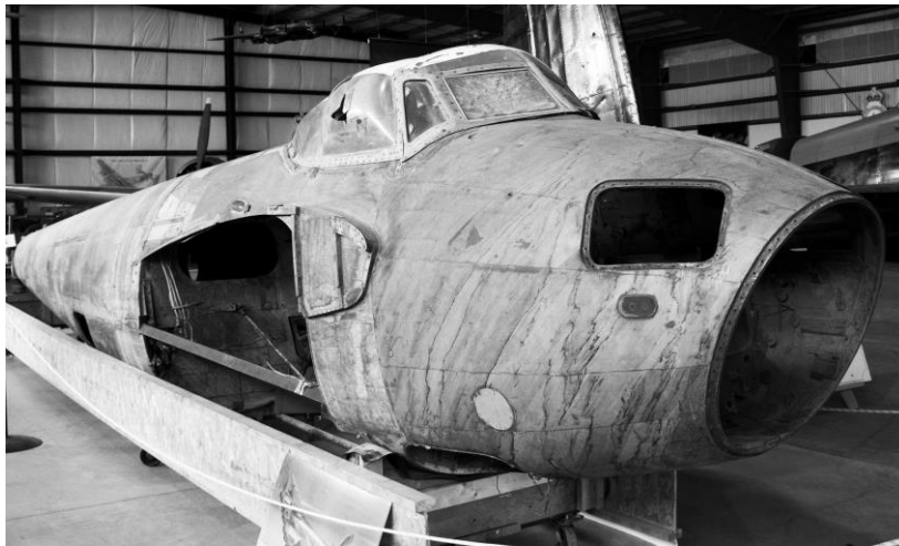
Figure 2.6: The wood fuselage of the “Mosquito” (Hisgett, 2012).
