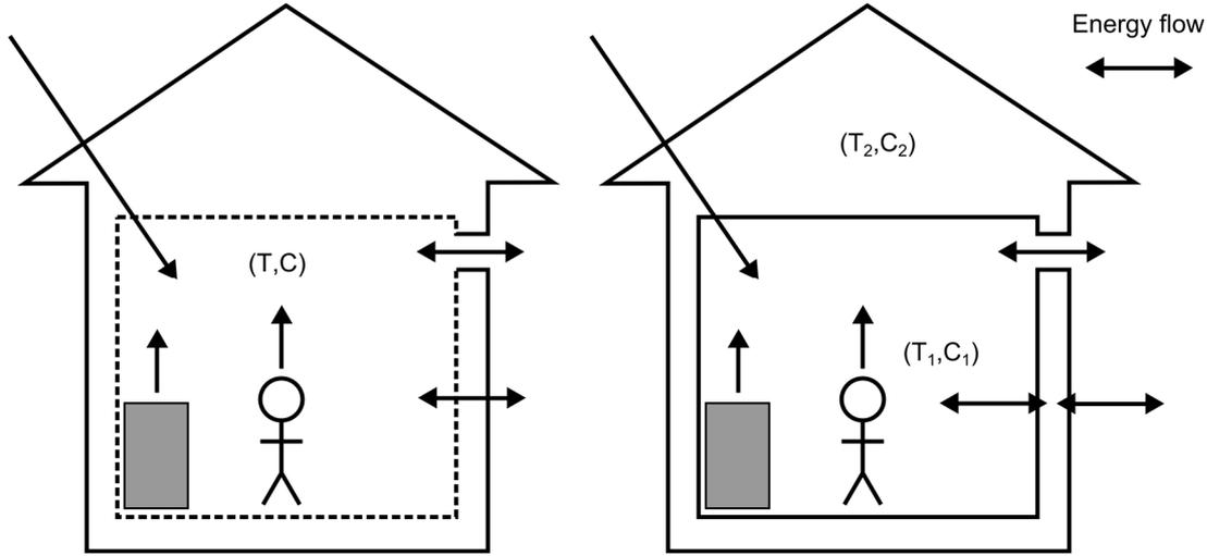
Figure 6. Conceptual description of the one-zone (left panel) and two-zone (right panel) energy balance models for a building. The arrows represent the different energy flows.
