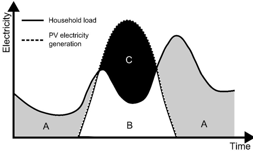
Figure 5. Conceptual description of a household load and PV electricity generation profile. A, The household load supplied by grid electricity; B, the household electricity supplied by PV-generated electricity; and C, PV-generated electricity fed to the grid.
