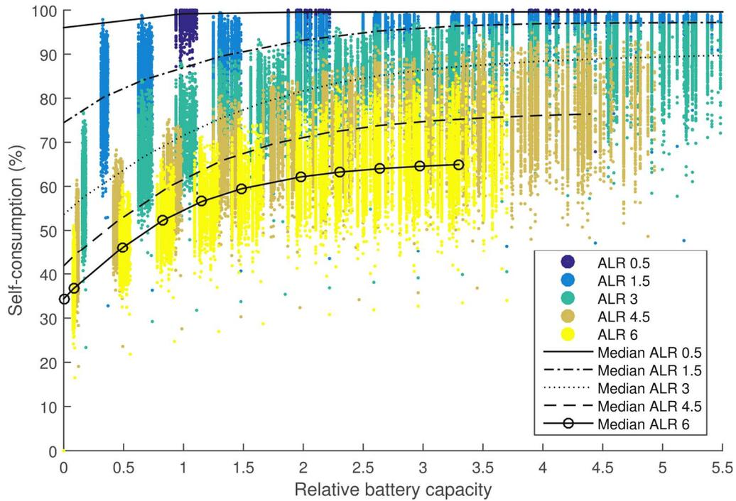
**Figure 10. PV electricity self-consumption (in percent) for four different ALRs, plotted against relative battery capacity. Each data-point represents a modeled household and the lines indicate the median value for the given ALR. Figure taken from Paper II.**
