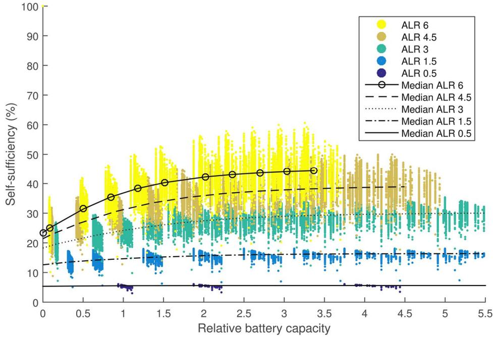
**Figure 9.** Self-sufficiency (in percent) for four different ALRs, plotted against the relative battery capacity. Each point represents a modeled household and the lines give the median value for the given ALR. Figure taken from Paper II.
