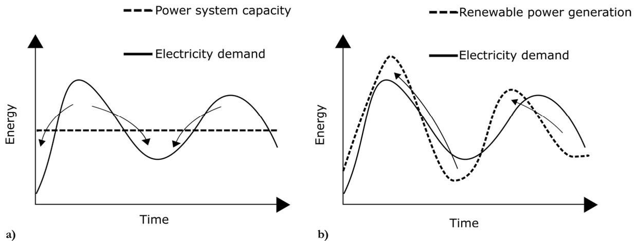
a) **Figure 2. Difference between demand response strategies in a traditional electricity system (a) and one with a considerable level of variable generation (b) [12]. The arrows represents the moving of demand.**
