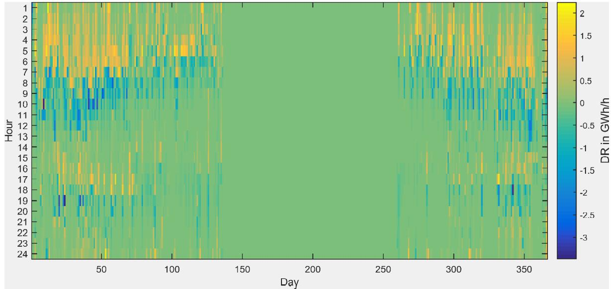
**Figure 18.** The hourly operation of DR for region SE2 in the DR case for the Green Policy scenario. The yellow coloration indicates an increase in load relative to the base case, and the blue coloration indicates a decrease in load relative to the base case. Adopted from Paper V
