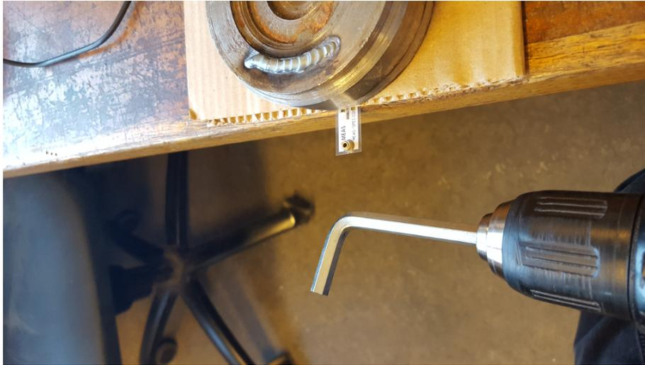
Figure 32: Drill used to excite piezo-electric material
