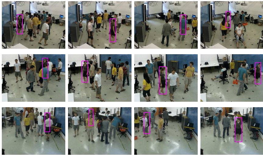
Figure 3.17: Tracking results of Method-6 in Case-f. Rows 1-3: Camera views 1-3. Key frames (# 3201, 3272, 3702, 3835) are selected.
