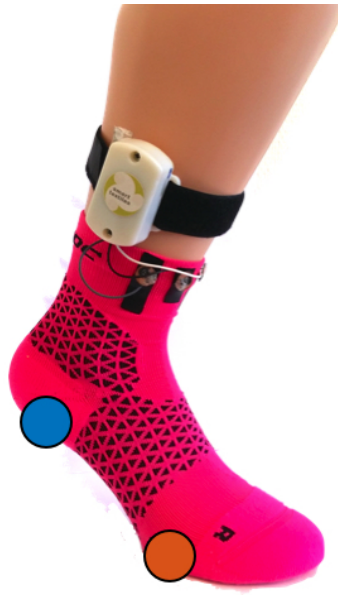
Figure 3.2: The blue circle marks the position of the heel sensor and the red circle marks the position of the toe sensor. The colors of the circles are the same ones used in plots throughout the report.
