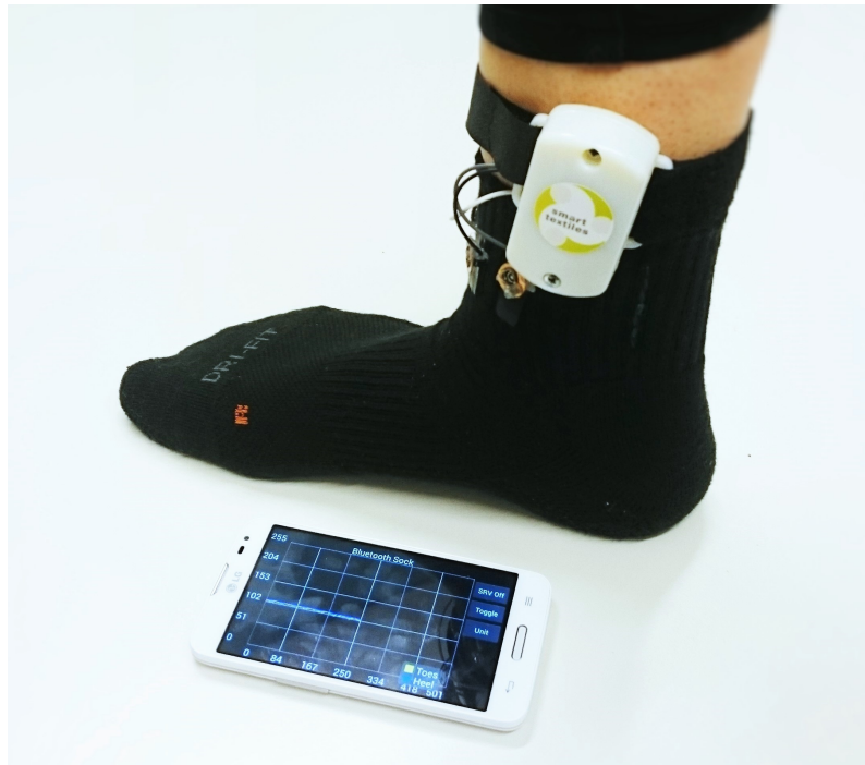
Figure 1.1: The current solution; the white box contains the blue-tooth unit and the phone shows the Android application with the time graph of the raw signals.
