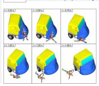
FIGURE 7 Illustration of the mechanical principle of influencing motion (left and middle) and occupant contact (right) <sup>12</sup>
