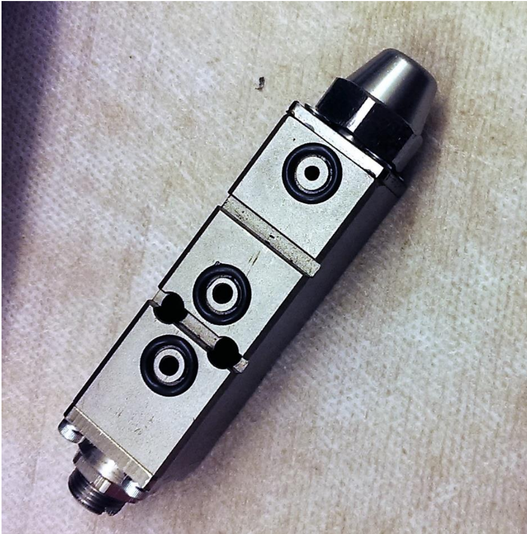
Figure 5. Glue-nozzle with O-rings that often replaces.
