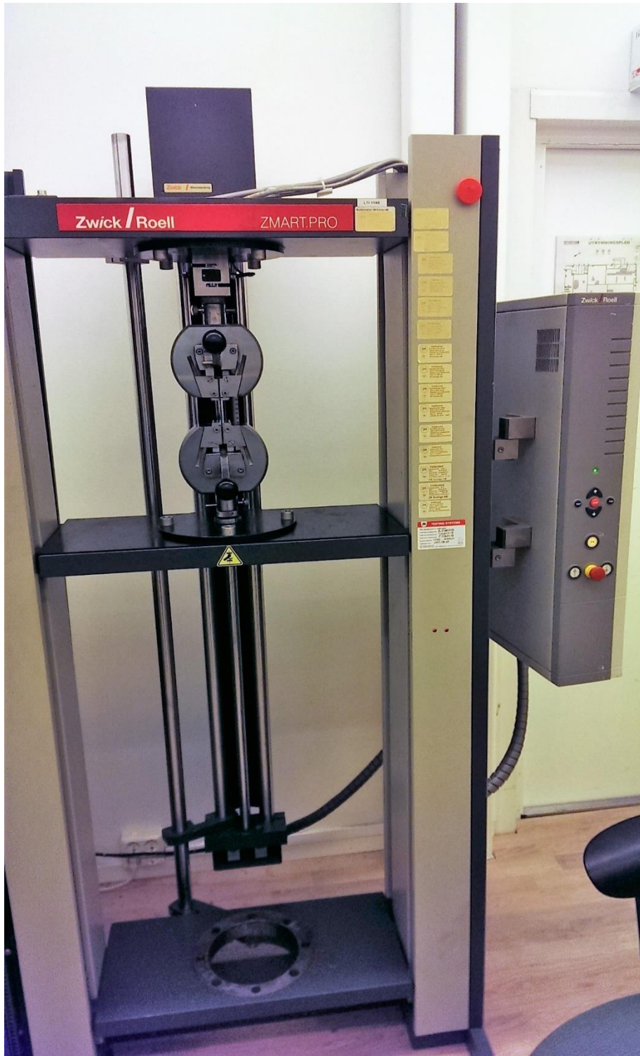
Figure 6. Pull test with operate panel on the right
