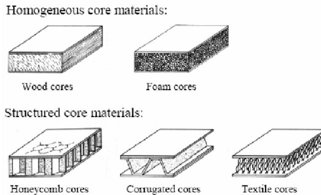
Figure 18. Different sandwich core types [19]
