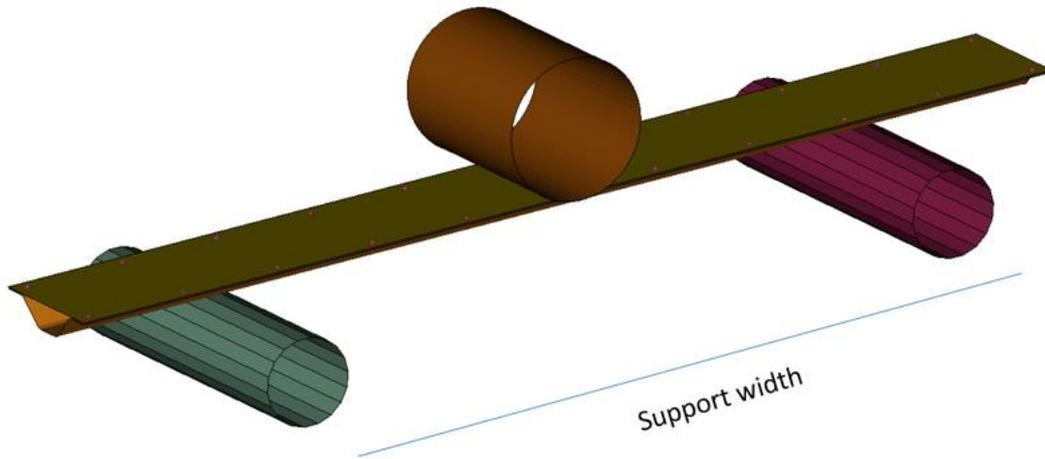
Figure 25. Illustration of the simulation in LS-DYNA. Representing the support widths
