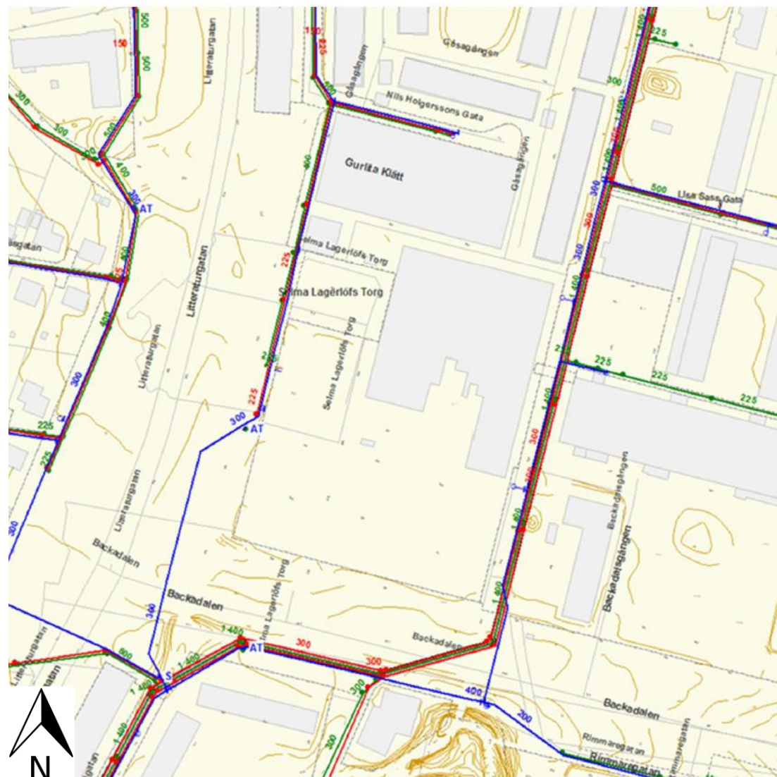
Figure 4.4 Existing water, sewage and stormwater pipes at Selma Lagerlöfs torg (Ramböll, 2013). Blue lines indicate water pipes, red lines represent sewage pipes and green lines are stormwater pipes.
