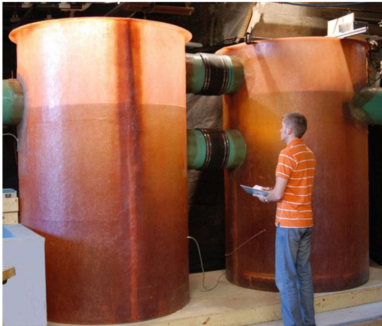
Figure 2.6 A full-scale two-chamber hydrodynamic separator (Source: Erickson et al., 2013a).
