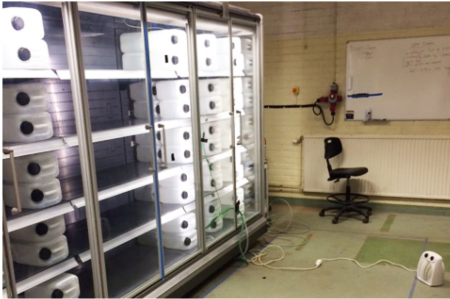
Figure 4.3: Photo showing the experimental setup with water filled canisters and one of the convective heaters.
