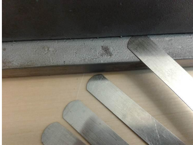
Fig. 3. Thickness gauges used to measure gap size.
