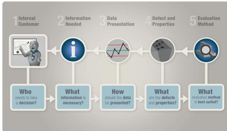
Figure 3: The PULL-approach model for evaluation of welds [1].
