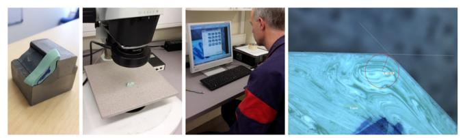
Fig. 6 WIA (weld impression analysis) used for evaluating the weld toe radius
