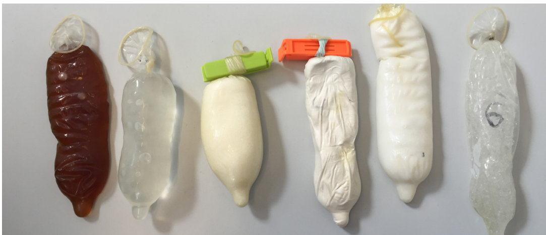
Figure 14.12: The oblong shaped models contained (from left to right) syrup, gel balls, sugar, flour, hair wax and crushed gel balls.
