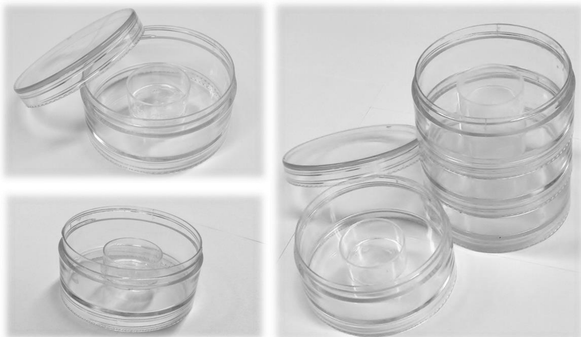
Figure 13. Pictures of homemade Conway cells used for the TVB-N experiment. Smaller jars are glued into larger jars. The larger jars are screwed on top of each other forming tight lids.
