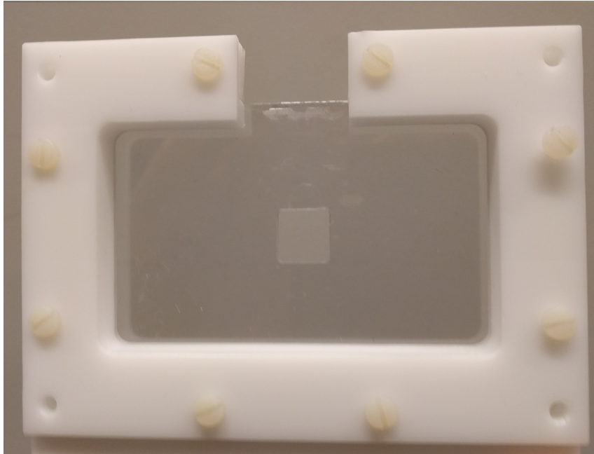
Figure 3.3: Image of the sample holder empty. The opening can be observed in the center of the holder.
