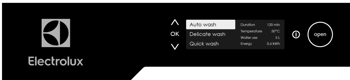
Figure 10.25 – The menu shows other available programs and information about the duration, temperature, water and energy use for the currently marked program
