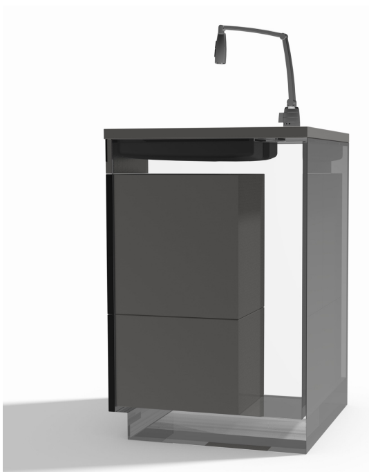
Figure 10.17 – The space available for the semi-tank and piping of the unit
