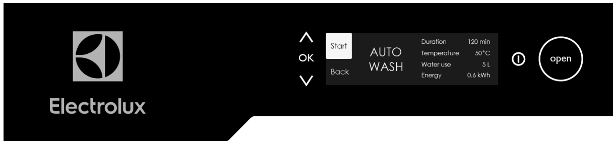
Figure 10.24 – The on/off button to the right has been pushed. The display shows a default auto wash program and information about its duration, temperature, water and energy use. The possible options are either to start the program or go back to the menu
