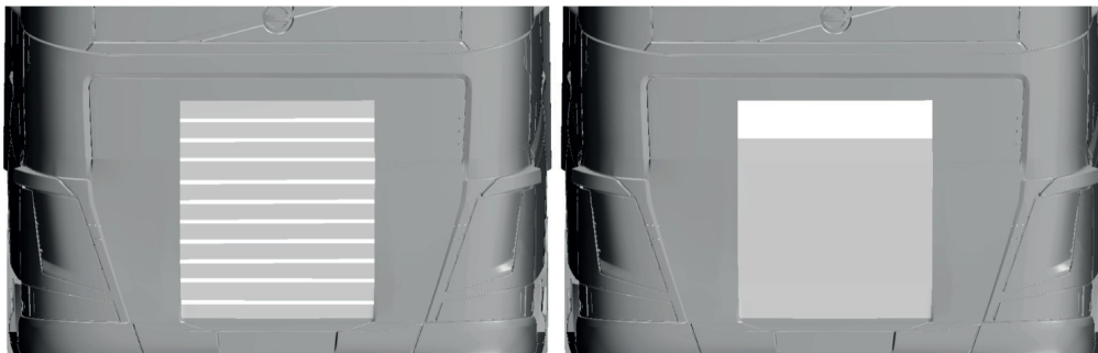
Figure 4.30: Approaches for the partially-opened grille-configurations. The HS are shown to the left, the CO to the right. The cases shown in the figure both corresponds to a grille opening percentage of 17.5%.
