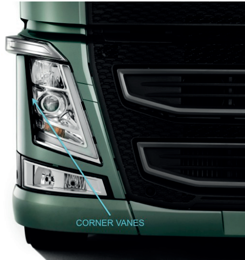
Figure 2.3: Corner vanes on a production type Volvo FH. The vanes are integrated with the head lamps [15].
